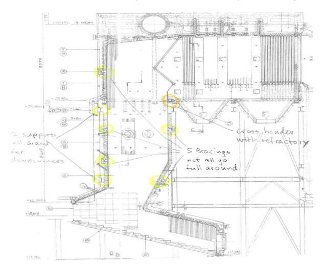
Existing probe port location can be found on drawings 324-4084 (Furnace front wall) and 324-4085 (Furnace back wall). Temperature probes are to be removed and replaced with new probes. Probes are as follows 6 probes- Moser TMTAG (AMK051-0320) and four probes (AMK-AF 051-0411) or equivalent.
