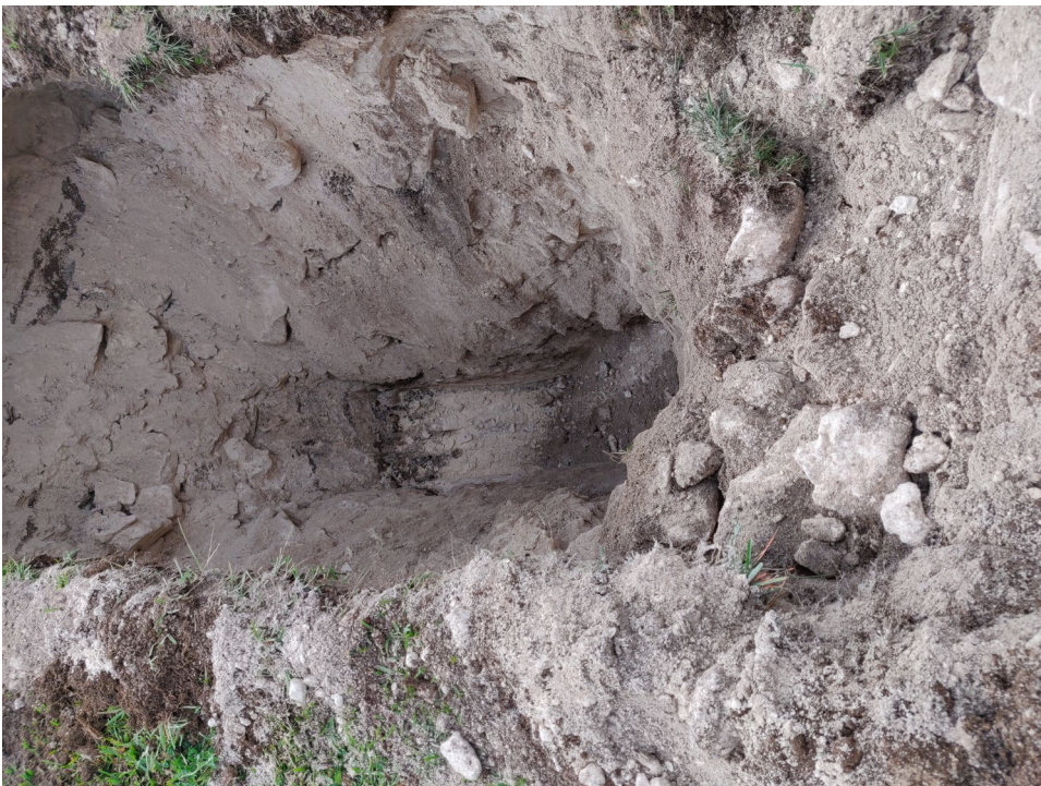
Trial Hole #2 – General fill down to rock
