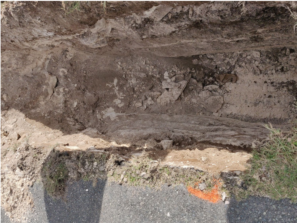
Trial Hole #3 – Rock level
